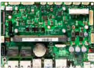
conga-SMC1/SMARC-x86 Carrier Board for x86 based SMARC 2.0 modules.
