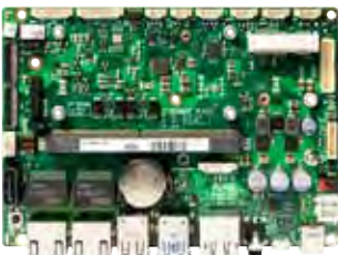
conga-SMC1/SMARC-ARM Carrier Board for ARM based SMARC 2.0 modules.
