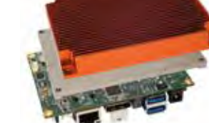
Cooler and heatspreader installed to bottom side of a Pico-ITX
