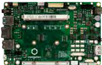
conga-MCB/ARM Small size (95x140mm) carrier board to support all ARM based Qseven modules.
