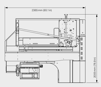
Machine height with safety cover closed 1990 mm (78.3 in) Machine height with safety cover open 2870 mm (113 in)
