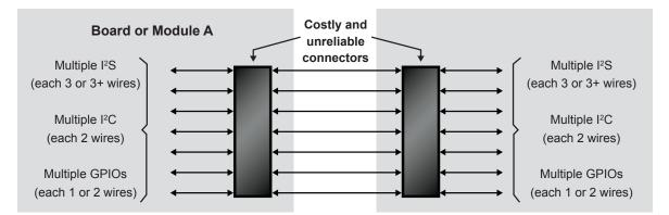
Figure 1: Traditional connectors are costly, consume space, and degrade the reliability of the system.
