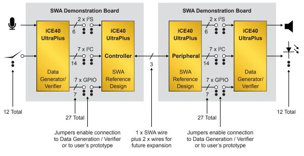
Figure 5: Block diagram of example SWA demonstration board setup.
