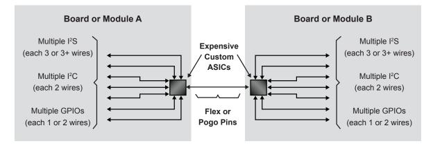
Figure 2: Custom ASICs are expensive, time-consuming to develop, and inflexible.
