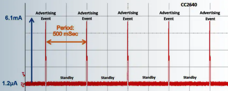
Figure 1: Current consumption versus time during a Bluetooth low energy advertising event.
