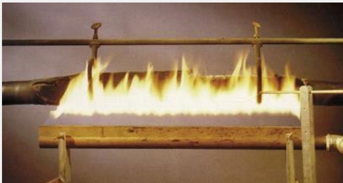
FIGURE 6: Fire-resistant joint before, during, and after a fire-resistant test. (TE connectivity)
