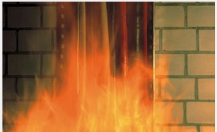
FIGURE 5: Flame-retardant heat-shrink cable accessories in a vertical tray arrangement. (TE Connectivity)
