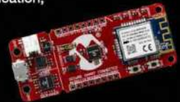
Figure 1: Microchip Technology AC164160 AVR-IoT WG Evaluation Board. (Source: Mouser Electronics)
