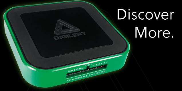
The Analog Discovery 3 is a digital oscilloscope, logic analyzer, waveform generator, pattern generator, and much more. Using the flexible WaveForms software (supported by Windows, Mac, and Linux), the Analog Discovery 3 can be used in the lab, in the field, or even at home - you're no longer tied down to a traditional benchtop and stacks of expensive test instruments.
