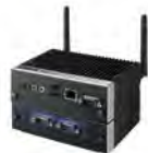
ARK-1124U Fanless Embedded Computer Intel Celeron N3350 Dual Core
