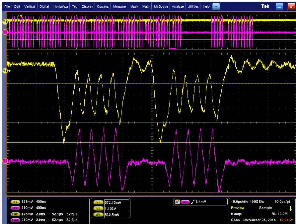
Figure 14- DDR4 Memory Lab Measurements with DDR4 Interposer
