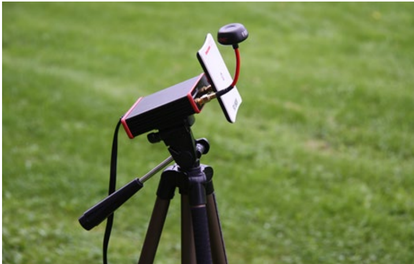
Fig. 5 Diversity Receiver with circular polarised antennas, one directional and one omnidirectional
