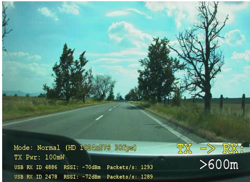
Fig. 11 Preserved video during reduced signal strength
