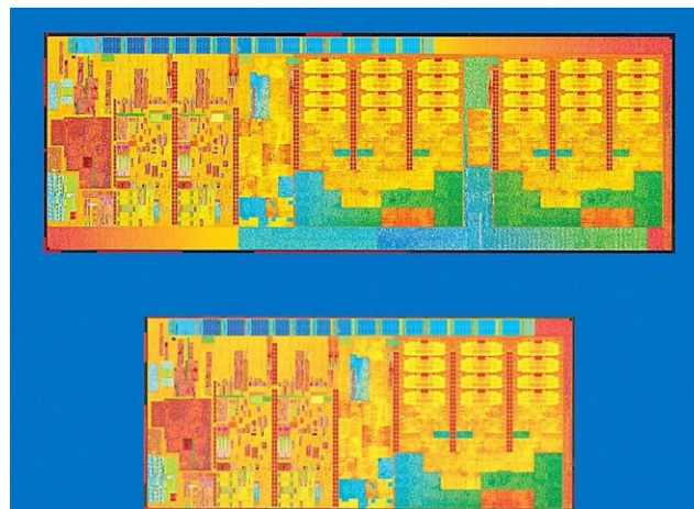
Haswell (top) and Broadwell (bottom). Die shrink in the transition from a 22nm to a 14nm process (source: Intel)
