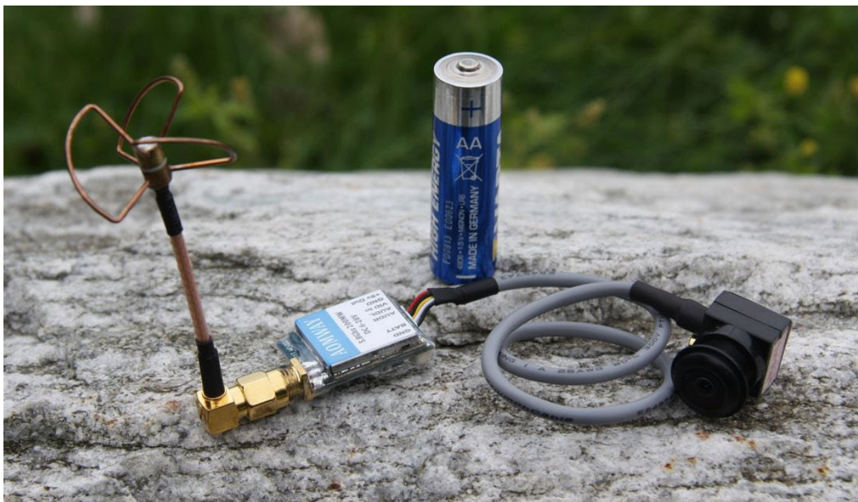
Fig. 7 Camera, analog transmitter and circular polarised antenna
